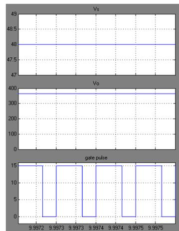
Fig. 6. Waveforms of input supply ( $V_s$ ), output ( $V_o$ ) and the gate pulse.
