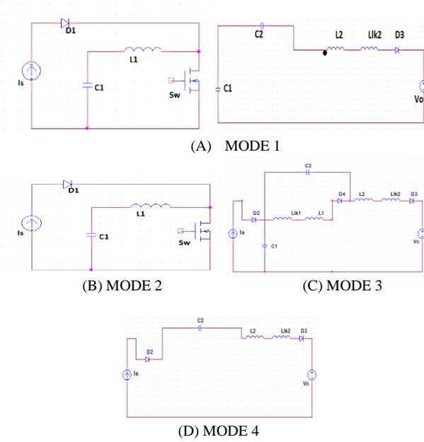
Fig. 3. Topological equivalent circuits cascaded boost converter.
