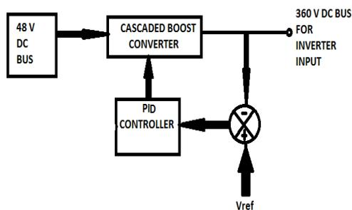
Fig. 1. Block diagram of cascaded boost converter.
