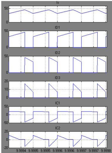
Fig. 7. Waveforms of the input current ( $I_s$ ), diode currents ( $I_{D1}$ ,  $I_{D2}$  &  $I_{D3}$ ) and the capacitor currents ( $I_{C1}$  &  $I_{C2}$ ).
