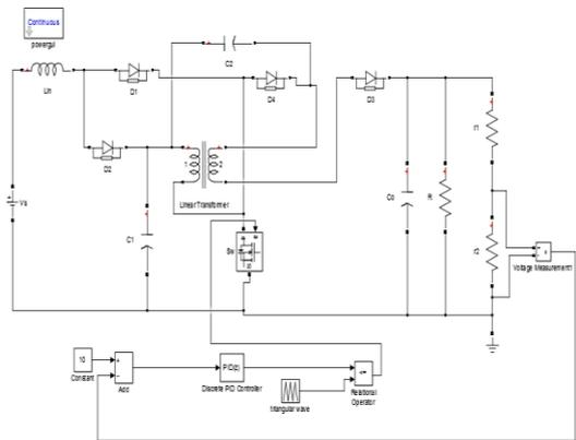
Fig. 5. Simulation circuit of cascaded boost converter.
