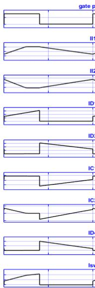
Fig. 4. Key waveforms of cascaded boost converter.
