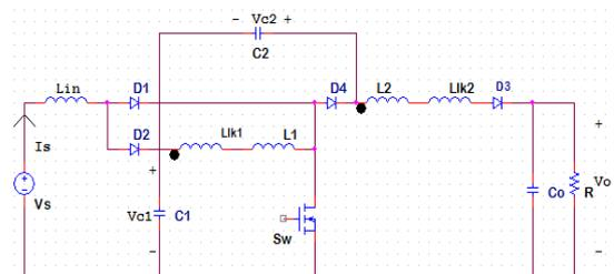
Fig. 2. Single switch cascaded boost converter.
