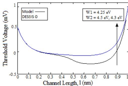
Fig. 6. Plot of surface potential v/s channel length plot for hafnium oxide dielectric obtained by varying work function  $w_2 = 4.5 \text{ eV}$ ,  $4.3 \text{ eV}$  and keeping  $v_{sb}=0 \text{ V}$ ,  $v_{gs}=0 \text{ V}$ ,  $v_{gb}=0 \text{ V}$ ,  $w_1 = 4.25 \text{ eV}$  and  $W_s=4.68 \text{ eV}$  constant.
