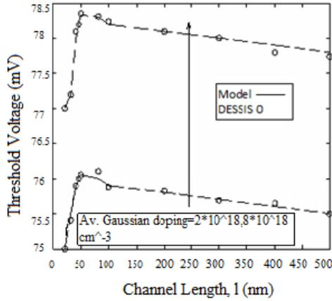
Fig. 4. Plot showing threshold voltage roll-off v/s channel length for  $n_{AV,GAUSS}=2*10^{18} \text{ cm}^{-3}$  and  $8*10^{18} \text{ cm}^{-3}$ .
