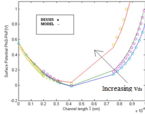
Fig. 3. The plot of surface potential versus channel length of dhdmg mosfet for three different values of the  $v_{ds}=0.25, 0.5$  and  $0.75$  V for  $l = 100$  nm and fixed doping of  $n_{SUB}=6*10^{17}$  cm<sup>-3</sup>,  $n_{AV,GAUSS}=6*10^{18}$  cm<sup>-3</sup> against the applied voltages  $v_{gs}=0v=v_{gb}=v_{sb}$ .
