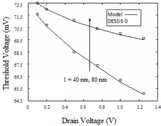
Fig. 5. Plot of threshold voltage v/s drain bias for a gaussian profile based dhdmg n-mosfet for  $v_{sb}=0 \text{ V}$ ,  $v_{ds}=0.5 \text{ V}$  for two different channel lengths,  $l=40$  and  $80 \text{ nm}$ , taking  $n_{SUB}=5*10^{17} \text{ cm}^{-3}$ ,  $n_{AV,GAUSS}=5*10^{18} \text{ cm}^{-3}$ ,  $l_p=10 \text{ nm}$ .
