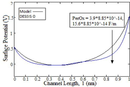
Fig. 8. Plot of surface potential v/s channel length for silicon dioxide and hafnium oxide obtained by varying oxide permittivity using  $\text{sio}_2$  permittivity  $= 3.9*8.85*10^{-14} \text{ f/m}$ ,  $\text{hfo}_2$  permittivity  $= 15.6*8.85*10^{-14} \text{ f/m}$  and keeping  $v_{sb}=0 \text{ V}$ ,  $v_{gs}=0 \text{ V}$ ,  $v_{gb}=0 \text{ V}$ ,  $w_1 = 4.25 \text{ eV}$ ,  $w_2 = 4.1 \text{ eV}$  and  $ws = 4.68 \text{ eV}$  constant.
