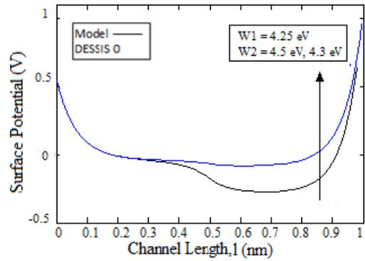
Fig. 7. Plot of surface potential v/s channel length plot for tantalum pentoxide dielectric obtained by varying work function  $w_2 = 4.5 \text{ eV}$ ,  $4.3 \text{ eV}$  and keeping  $v_{sb}=0 \text{ V}$ ,  $v_{gs}=0 \text{ V}$ ,  $v_{gb}=0 \text{ V}$ ,  $w_1 = 4.25 \text{ eV}$  and  $W_s=4.68 \text{ eV}$  constant.
