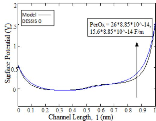
Fig. 9. Plot of surface potential v/s channel length for  $\text{hfo}_2$  and  $\text{ta}_2\text{o}_5$  obtained by varying oxide permittivity using  $\text{ta}_2\text{o}_5$  permittivity  $= 26*8.85*10^{-14} \text{ f/m}$ ,  $\text{hfo}_2$  permittivity  $= 15.6*8.85*10^{-14} \text{ f/m}$  and keeping  $v_{sb}=0 \text{ V}$ ,  $v_{gs}=0 \text{ V}$ ,  $v_{gb}=0 \text{ V}$ ,  $w_1 = 4.25 \text{ eV}$ ,  $w_2 = 4.1 \text{ eV}$  and  $W_s=4.68 \text{ eV}$  constant.
