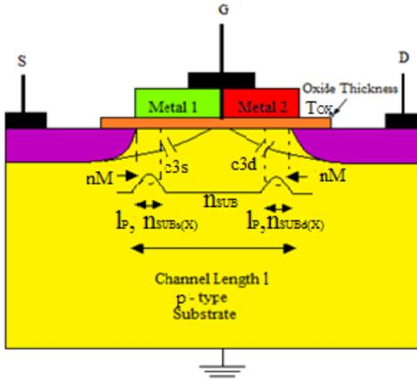
Fig. 1. Structure of n-channel gaussian doped dhdmg mosfets.
